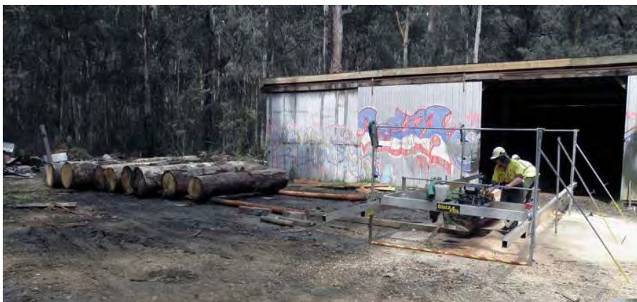
Set-up of the Lucas Mill at the Parks depot
