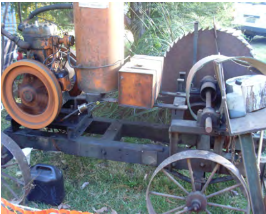
I have worked on our old 4hp Ronaldson Tippet petrol engine. It is now up and running, with a new Champion D21 spark plug.
